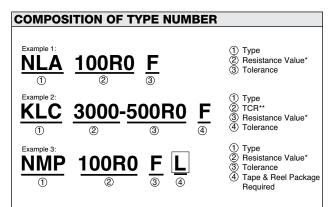
\*Resistance value, in ohm, is expressed by a series of five characters, four of which represent significant digits. R or K is a dual-purpose letter that designates both the value range (R for ohmic; K for kilo-ohm) and the location of decimal point.
