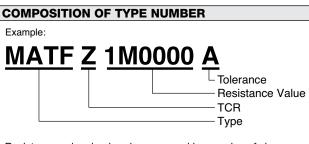
Resistance value, in ohm, is expressed by a series of six characters, five of which represent significant digits. K or M is a dual-purpose letter that designates both the value range (K for kilo-ohm; M for mega-ohm) and the location of the decimal point.
