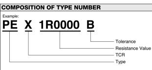
Resistance value, in ohms, is expressed by a series of six characters, five of which represent significant digits. R or K is a dual-purpose letter that designates both the value range (R for ohmic; K for kilo-ohm) and the location of the decimal point.
