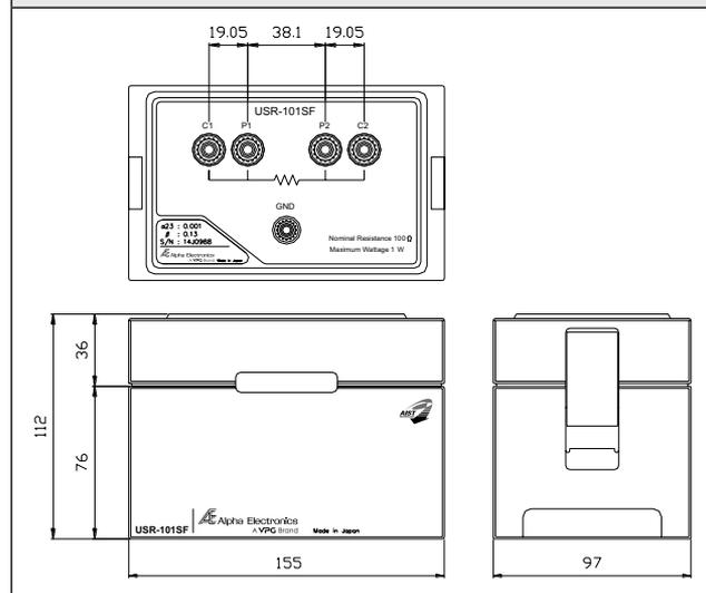
The resistive elements are held by special designed case so, it's suitable for environment with vibration during transportation.
