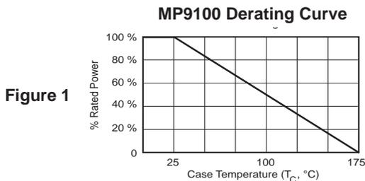
In high power applications, the actual power dissipation capability of the resistor will be greatly dependent on the heat sink, mounting method, interface
