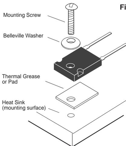
Figure 2 MP9100 with Mounting Screw and Belleville Washer
