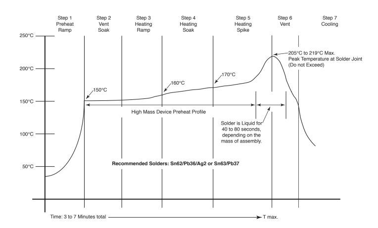
**Do Not Exceed 219°C when soldering.** Caddock Model MP725 and Type CD resistors (and some custom SMT resistor products) contain internal solder connections made with Sn/Ag solder (melts at 221°C).
