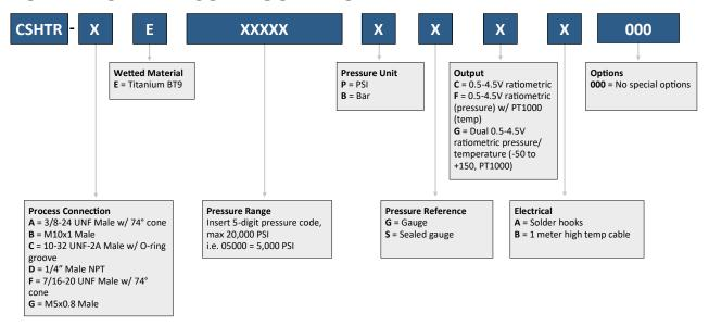
Ordering Example: CSHTR-AE01000BSCA000 (3/8-24 UNF Male w/ 74° cone, Titanium BT9, 0-1000 Bar sealed gauge, 0.5-4.5V ratiometric, Solder hooks)
