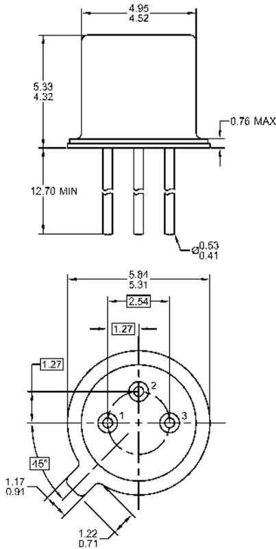
1. All linear dimensions are in millimeters.
