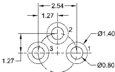
1. All linear dimensions are in millimeters.
