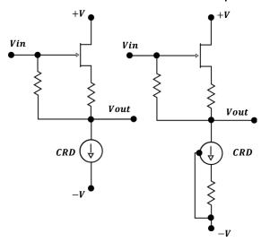
When the resistor values are selected properly to allow operation at about VGS = VGS(off) – 0.63 V for the CRD and VP + 0.7V for the JFET, the circuit will have a near Zero-Temperature Coefficient (Zero-TC). This means that the device will vary minimally with changes in temperature.
