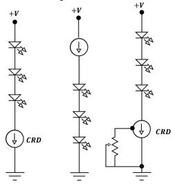
The maximum number of LEDs is determined by adding the voltage drop across the LEDs and the CRD. Add the current requirements for each LED to select the correct CRD from the data sheet.
