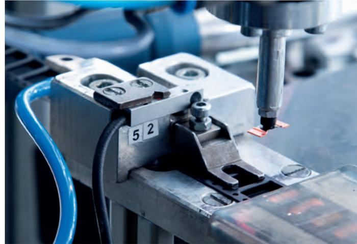
Components are comprehensively tested, measured and calibrated before packing in standard tapes and reels
