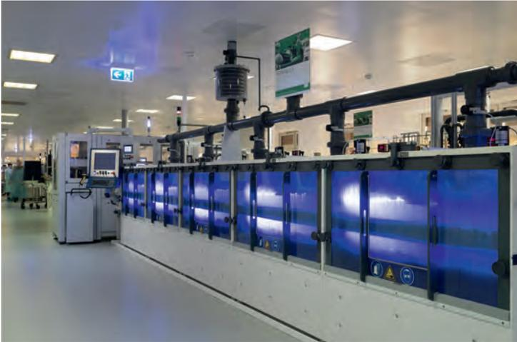
Etching technology process of ISA-PLAN® resistors
