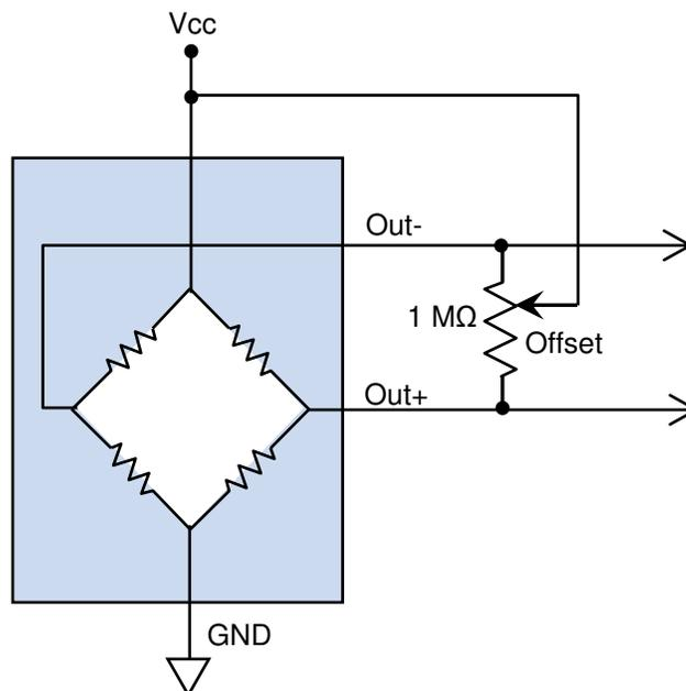
**Figure 2. Offset correction with a potentiometer.**
