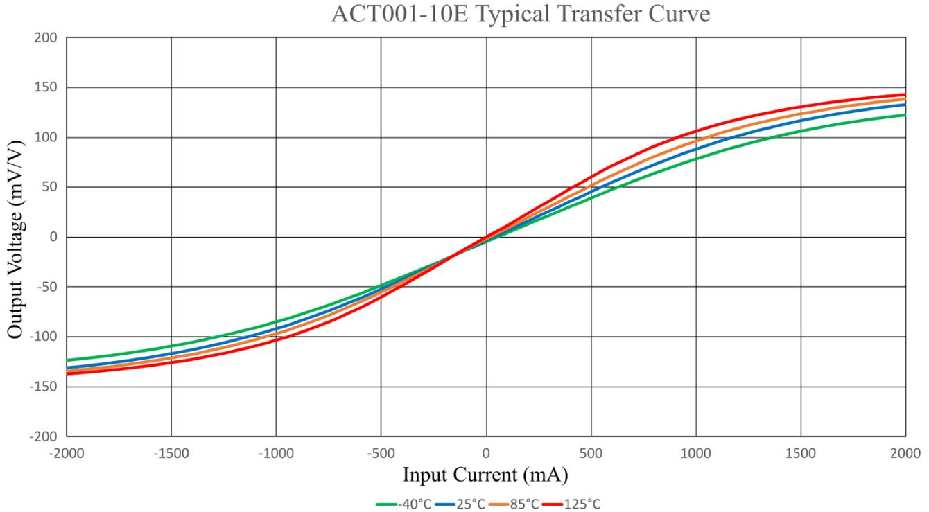
**Figure 1: Typical ACT001 operating characteristic over temperature.**
