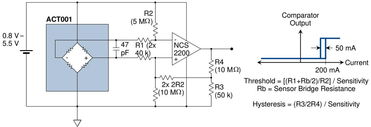
**Figure 5. Overcurrent comparator circuit with hysteresis.**
