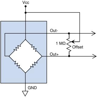
Figure 2. Offset correction with a potentiometer.NVE Corporation• 11409 Valley View Road, Eden Prairie, MN 55344-3617• (952) 829-9217• www.nve.com
