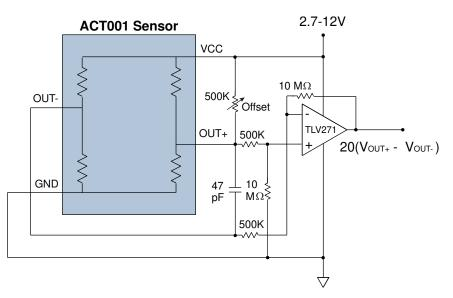
Figure 3. Differential amplifier circuit.
