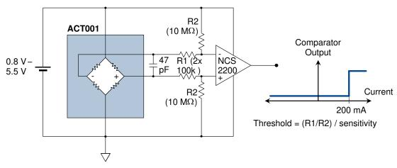
Figure 4. Single-comparator overcurrent circuit.
