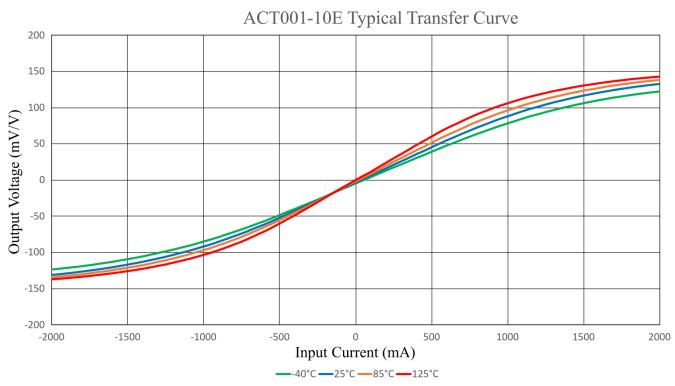
Figure 1: Typical ACT001 operating characteristic over temperature.
