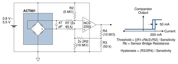
Figure 5. Overcurrent comparator circuit with hysteresis.
