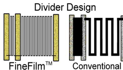
The long serpentine pattern used in manufacturing Fine Film Dividers (HVD's), coupled with the use of low Ohms/square thick film inks, makes it possible to create virtually any divider ratio with exceptional tracking. For example, OhmCraft has produced 800 Meg-Ohm dividers with a 20,000:1 ratio. Low noise, low TCR, low VCR, and many other features add up to the finest leaded divider in the industry today.
