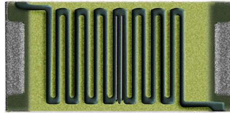
These components have been designed and tested especially to withstand and dissipate very high peak voltage energy pulses and transient overloads using FineFilm™ thick film technology. They are especially effective by comparison with conventional designs in higher values. In order to maximize these advantages they are usually designed without close tolerance features such as trim areas.
