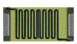
These components have been designed and tested especially to withstand and dissipate very high peak voltage energy pulses and transient overloads using FineFilm<sup>™</sup> thick film technology. They are especially effective by comparison with conventional designs in higher values. In order to maximize these advantages they are usually designed without close tolerance features such as trim areas.
