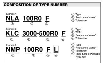
\*Resistance value, in ohm, is expressed by a series of five characters, four of which represent significant digits. R or K is a dual-purpose letter that designates both the value range (R for ohmic; K for kilo-ohm) and the location of decimal point.
