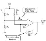
$$V_{OUT} = \left(\frac{R_2}{R_1 + R_2} - \frac{R_1}{R_1 + R_2} \times \frac{R_4}{R_3}\right)_{x} V_{dd}$$
