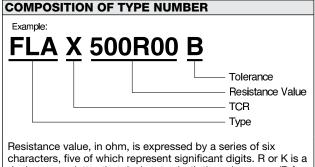
characters, five of which represent significant digits. R or K is a dual-purpose letter that designates both the value range (R for ohmic; K for kilo-ohm) and the location of decimal point.
