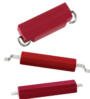
their normally-open resting state. Higher AT/less sensitive switches have a wider contact gap, requiring greater blade deflection to close the gap. This greater deflection creates stronger springback forces in the blades when the magnet is removed, thereby pulling the blades apart more forcefully than with a low AT/more sensitive switch.
