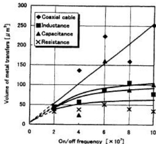
Fig. 6. Dependence of the volume of bumps of transferred Ru metal on R,C,L and coaxial cable as circuit loads as a function of on/off frequencies.
