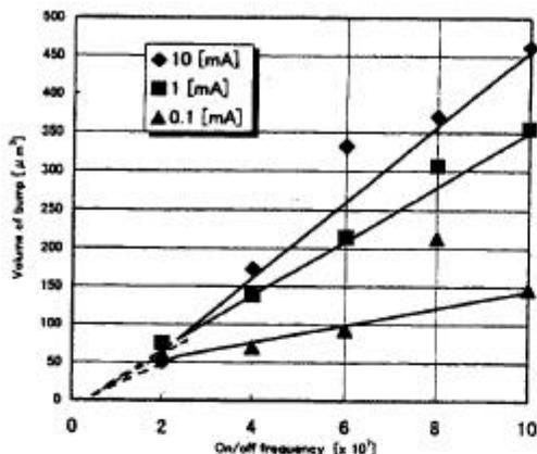
Fig. 5. Volumes of bumps for transferred Rh 2 metal versus on/off frequencies.
