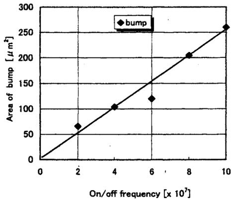
Fig. 2. Bump areas for transferred Rh 1 metal plotted against on/off frequencies.
