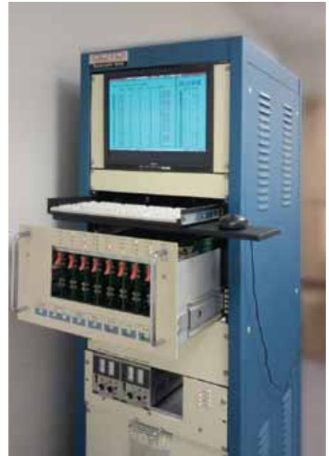
Each system has 32 test channels capable of testing reed switches at loads that can be varied from 0.03V, 1mA (30 microwatts) to 60V, 1A (60 watts). Auxiliary driver modules allow loads up to 150V, 10A
