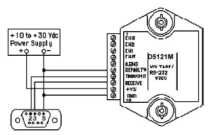
Note: If using a DB-25 connector ground is tied to pin 7. Pin 3 is tied to TRANSMIT and pin 2 is tied to RECEIVE on the module.
