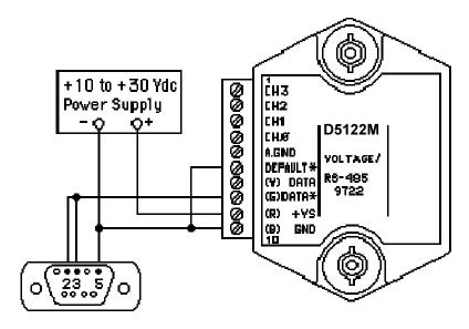
Note: If using a DB-25 connector ground is tied to pin 7.
