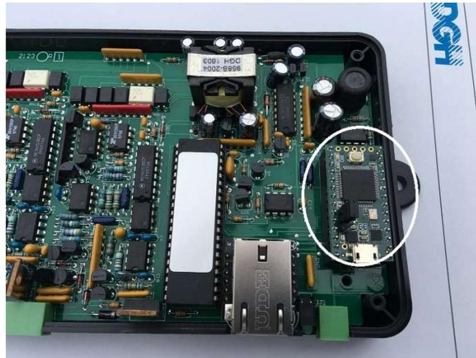
5. Move the jumper from the back two pins to the front two pins as seen in the picture below.
