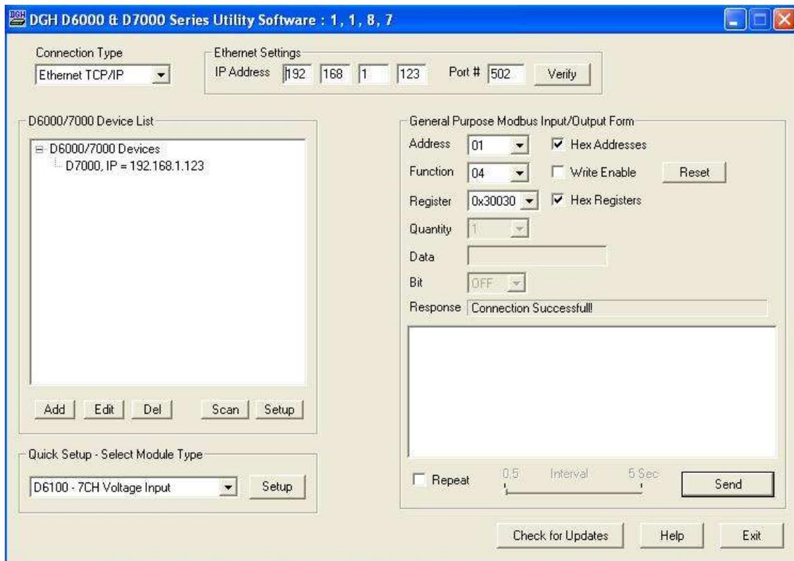
After a successful connection test has been performed then the module can be configured. Select the type of module using the drop-down list box under “Quick Setup” in the lower left hand corner of the screen. Then press the “Setup” button and a new screen (see below) will appear that contains list of all the user-selectable module values. Several different screens will appear for the different types of module that are connected. The screen below is for a seven channel current input module.
