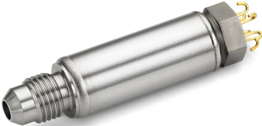
The Paine 211-50-070 Series is our rugged High Pressure/High Temperature (HP/HT) combination transducer designed for +500 °F (+260 °C) offshore oil, gas, and power industry requirements. The Paine 211-50-070 Series, based on its small size, all-welded construction, and ability to perform in corrosive high shock and vibration environments, is the best solution for new tool and process equipment design when temperatures are going to reach +500 °F (+260 °C).
