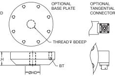
NOTES: 1. 100 LB THRU 5000 LB UNITS ARE COUNTER-BORED FOR SOCKET HEAD CAP SCREWS. 2. OPTIONAL THREAD STOPS ADDED IN LOAD CELL WHEN ORDERED WITH BASE KIT.
