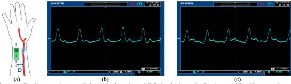
Fig. 4. Displacement ( $D$ ) of sensor unit w.r.t. radial artery is shown in (a). MPG signals observed at  $D = 0$  mm and  $D = 25$  mm are shown in (b) and (c).
