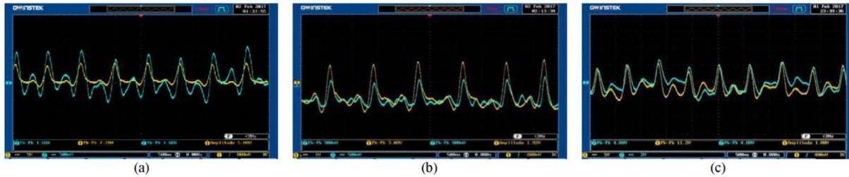
Fig. 7. MPG signals showing Pulse Transition Time for three different volunteers.
