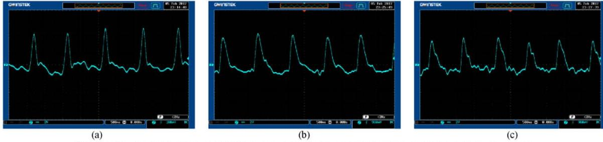
Fig. 5. MPG waveforms observed at Wrist, Lower Arm, and Upper Arm are shown in (a), (b) and (c) respectively.
