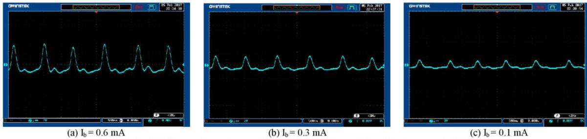
Fig. 6. MPG waveforms observed for a volunteer at three different biasing current ( $I_b$ ).
