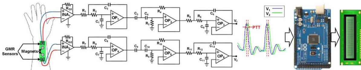
Fig. 1. Schematic Diagram of the developed Prototype showing typical PTT for a volunteer and detailed analog conditioning circuit.
