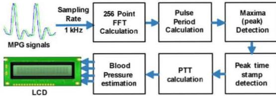
Fig. 2. Block diagram of Blood Pressure estimation algorithm.
