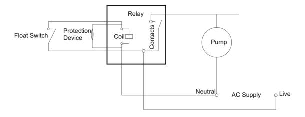
It is advisable to fit a 375V bi-directional Transil across the relay coil terminals, if the control voltage is 240Vac.
