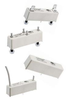
Recently approved by UL, very high isolation voltages (up to 10kV) are achieved through the use of high vacuum reed switches with either rhodium or tungsten contacts and make these relays suitable for high reliability applications, such as cardiac defibrillators, test equipment and high voltage power supplies.
