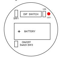
Switches 1, 2, 3 & 4 select the RF Network the IWTT will transmit on. The default network for both the IWTT transmitter and IWR receiver is network 1.
